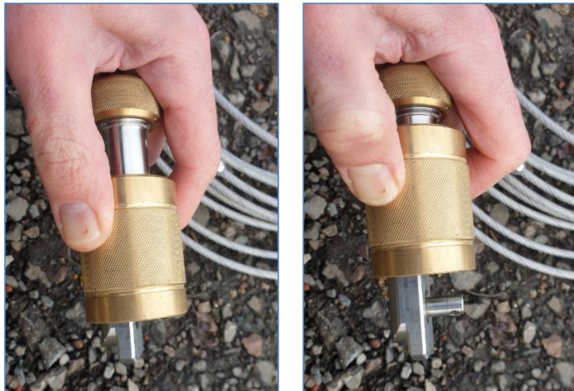
Figure 43 Deployment adaptor with brass cuff un-retracted (left) & retracted (right)
