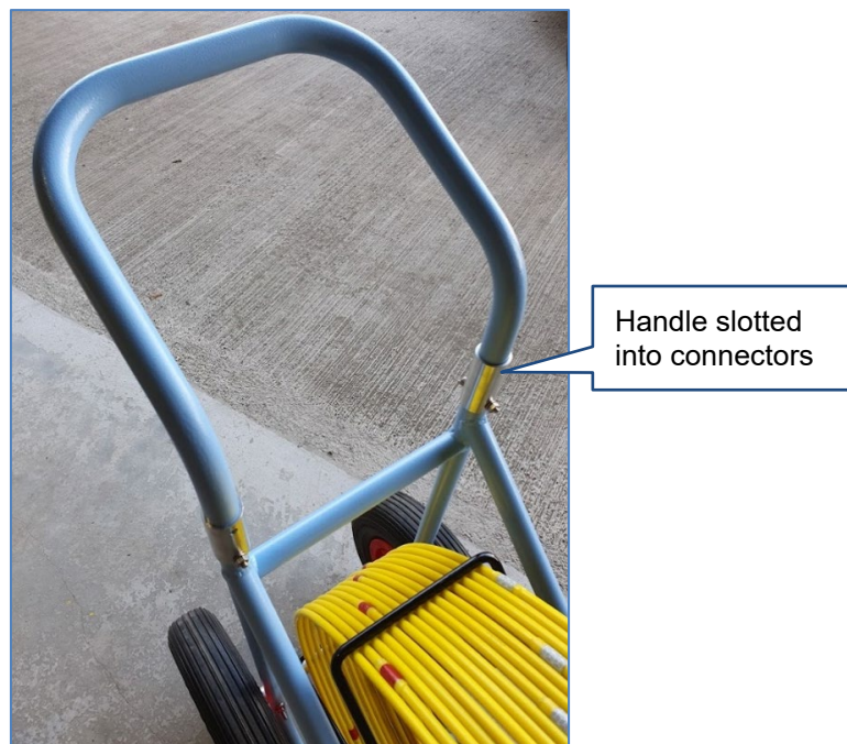
Figure 57 Assembling the push rod system - step 6
