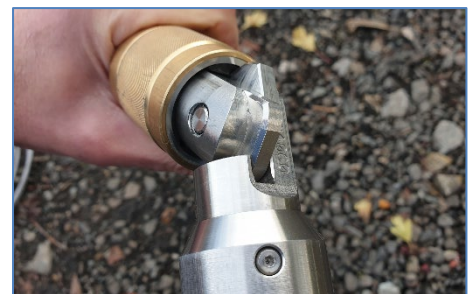
Figure 45 Retracted deployment adaptor ready to connect to the probe
