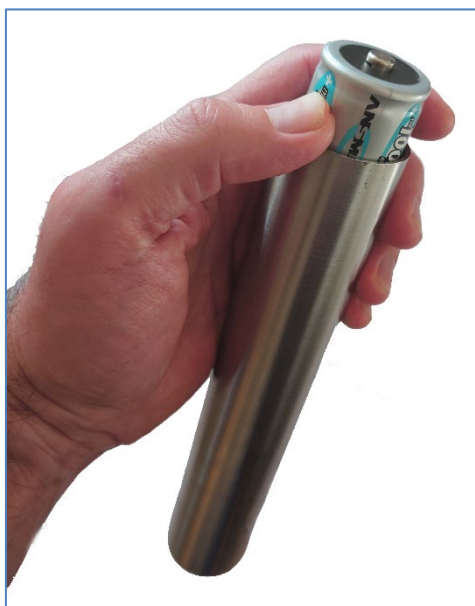
Figure 35 Positive battery terminals face out
