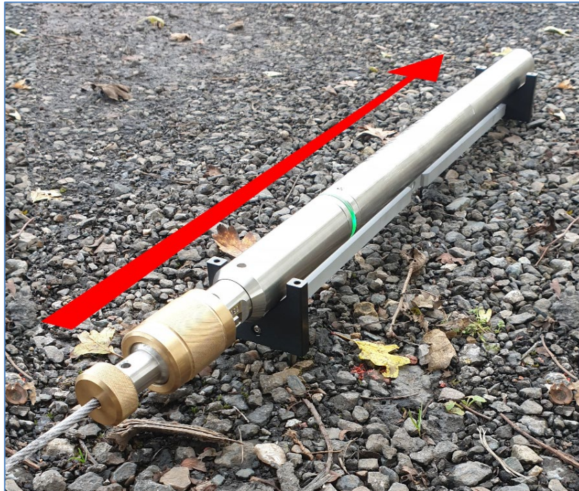
Figure 2 Surveyed heading of the alignment jig
