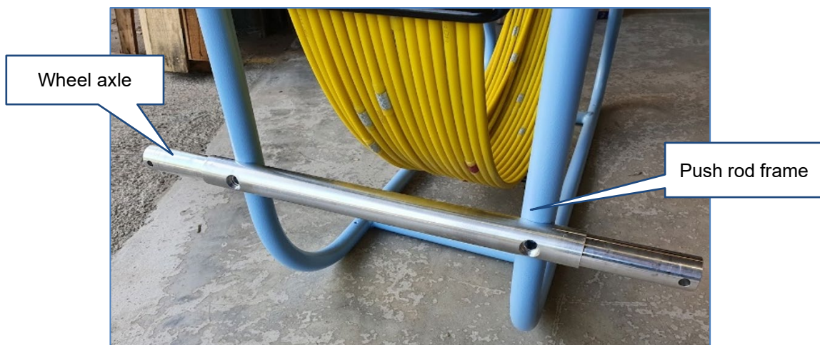
Figure 53 Assembling the push rod system - step 2
