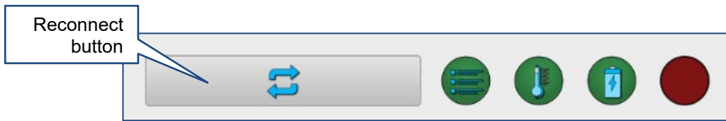
Figure 125 Probe status when alignment has been lost
