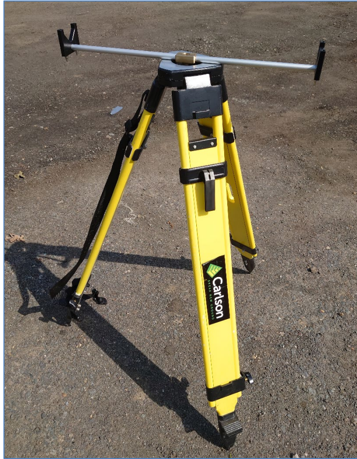
Figure 41 Gyro alignment jig mounted on a survey tripod
