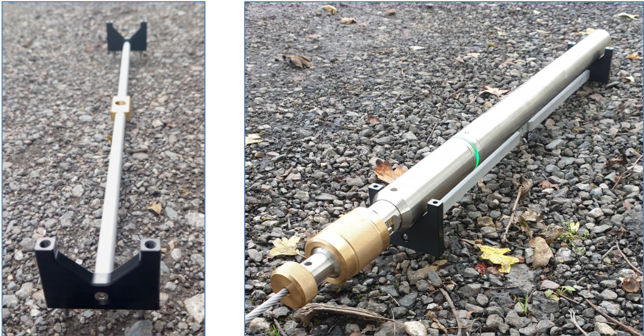
Figure 40 Gyro alignment jig (left) with probe during alignment (right)
