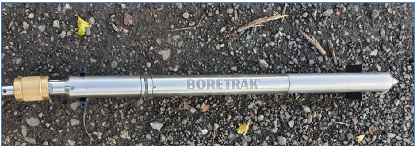
Figure 12 Probe held in the alignment jig
