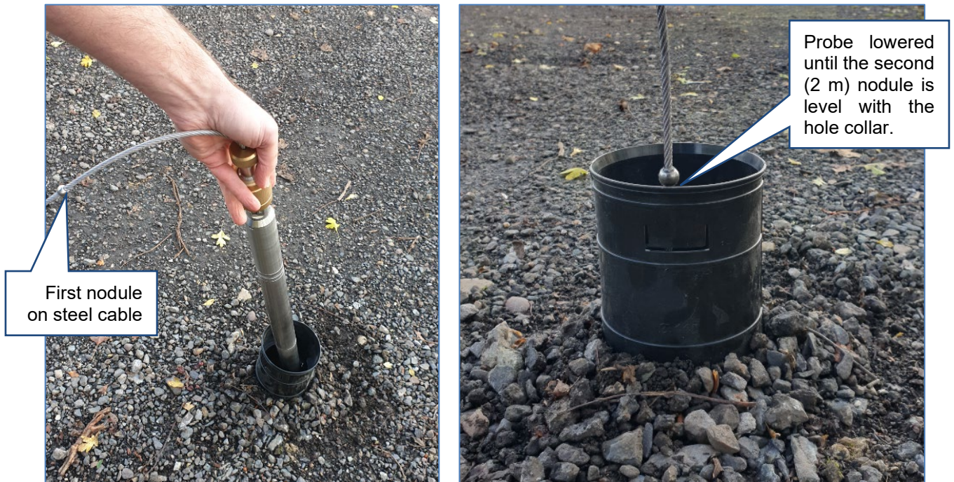
Figure 19 Deploying the probe into the hole
