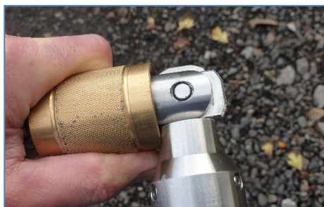
Figure 44 Connecting the deployment adaptor to the probe
