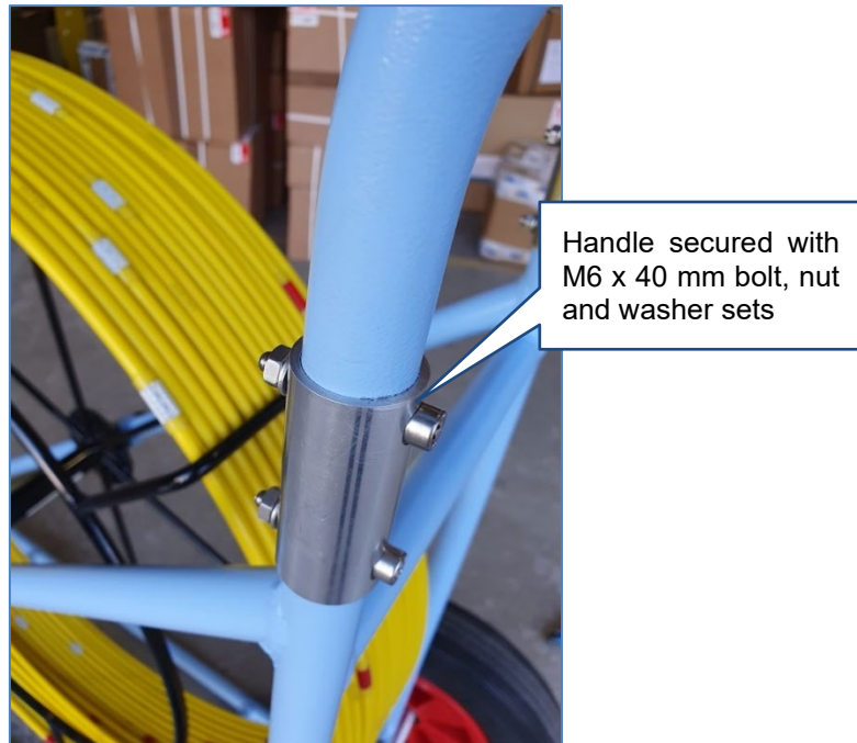
Figure 58 Assembly of the push rod system - step 7
