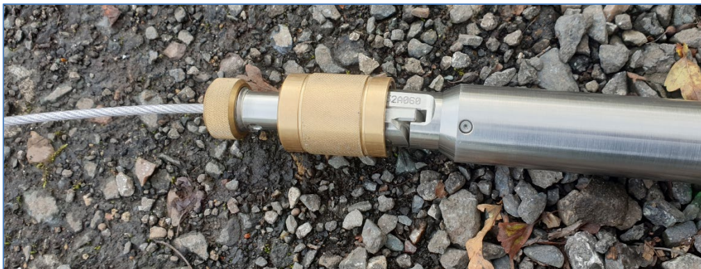
Figure 46 Deployment adaptor connected to the probe
