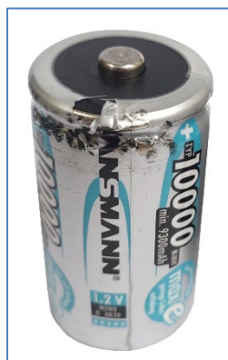
Figure 36 An example of a battery with a damaged outer coating. This battery should not be used in the Boretrak2 probe
