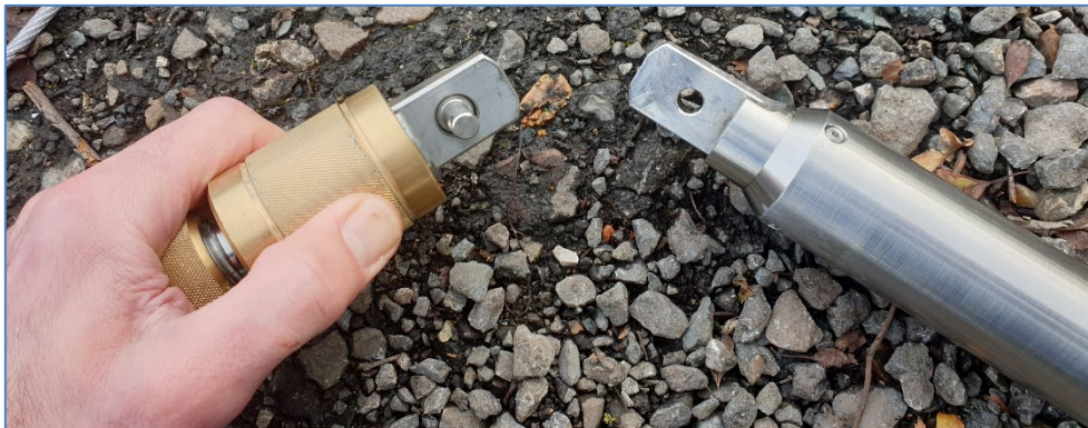
Figure 45 Retracted deployment adaptor ready to connect to the probe
